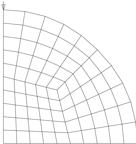
Figure 11.1: Mesh for Circular Disk. 75 Elements
