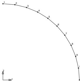
Figure 5.2: Mesh for Curved Beam. 10 Elements
