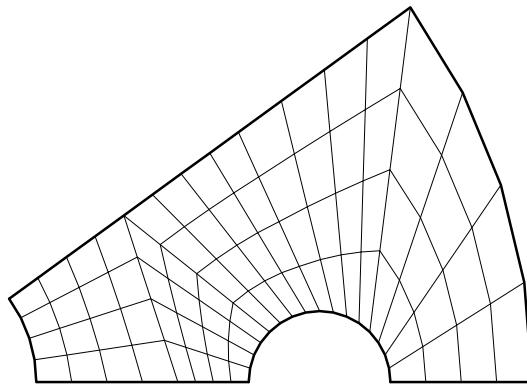
Figure 5.10: Mesh segment for disk with holes
