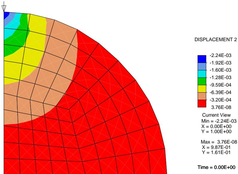
Figure 11.2: Contours of Vertical Displacement for Circular Disk
